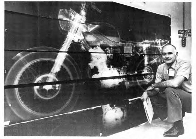
BILL MOTTERN, Radiography project leader for the Area III Nondestructive Testing Laboratory, displays x-ray of motorcycle, taken to show capability of the Lab. Source for the image was a mobile 10 MeV x-ray machine designed to Sandia specifications.
